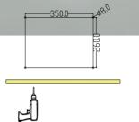
Use an electric drill to drill four  $\phi$   $\Phi$ 8mm holes in the ceiling according to the size of 270x220mm.
